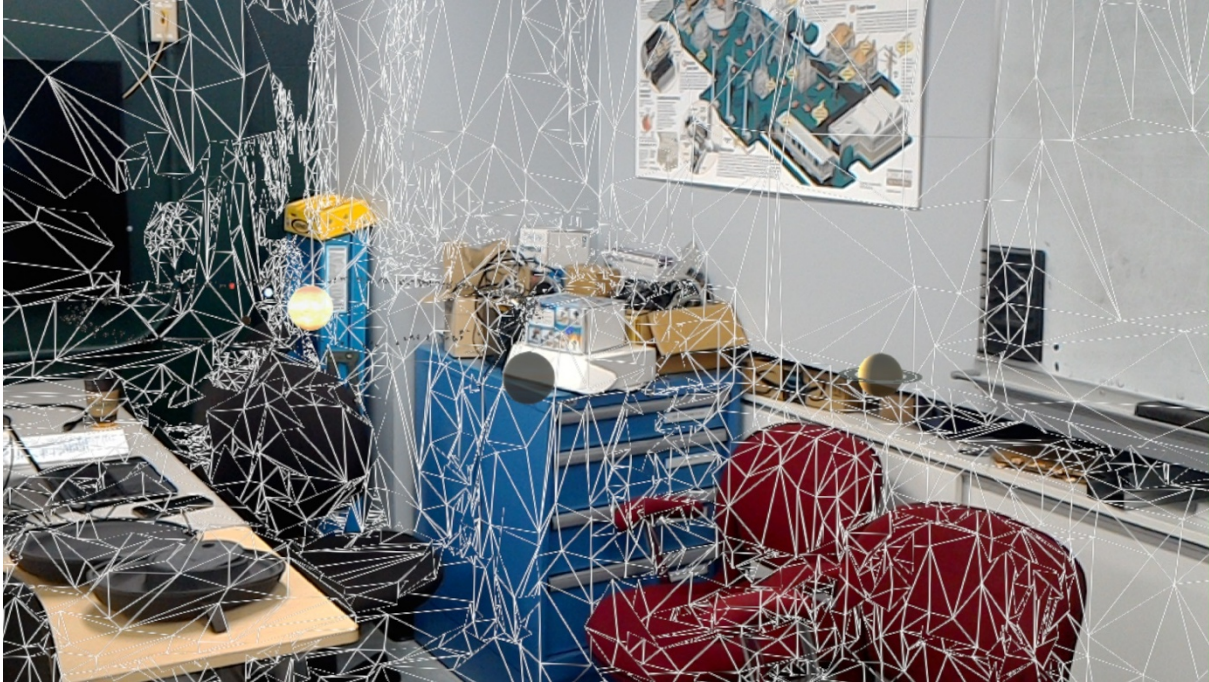
Figure 32: Microsoft HoloLens displaying a real-time mesh layout when we deploy a project with the SpatialMapping.cs script with grid enabled
