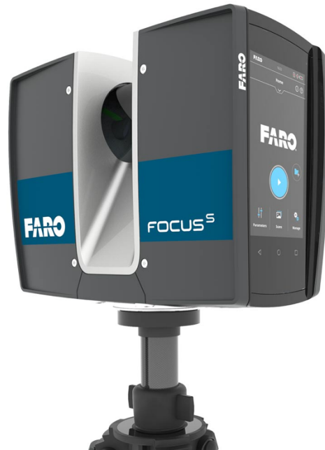
Figure 3: FARO's LIDAR scanner device
